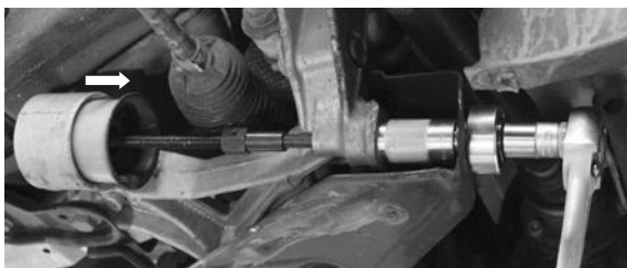
Fig. 4 Extracting the silentbloc
