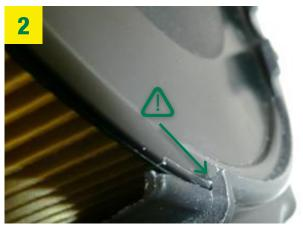
Ensure that the edge of the element base completely fits into the groove of the housing.
