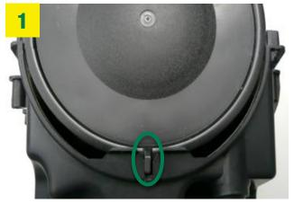
When inserting the filter element, ensure that the alignment contour is correctly placed into the notch provided.
