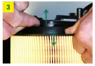
Pull the housing wall away from the element and at the same time pull the element in the opposite direction. Press the flexible seal over the lip of the housing.
