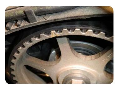
**4.** Remove the timing covers and slacken the tensioner. Then remove the timing belt and water pump. Ensure that the water pump area is clean, then fit the new VKPC 86810 water pump and torque to the manufacturers' recommendations.
