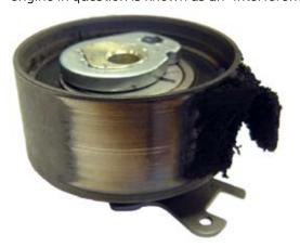
type engine. This means that in the event of timing belt failure, valve to piston damage will occur. When it comes to the scheduled servicing of the timing system, vehicle manufacturers' guidelines should always be followed.
