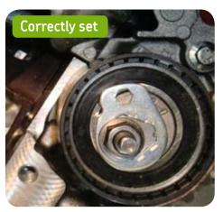
**Caution:** If the tensioner is touching the cylinder head the procedure must be restarted.
