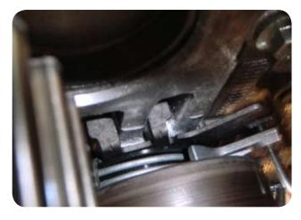
**5.** Ensure the locating pegs on the VKM 16002 tensioner are correctly positioned in the engine block.
