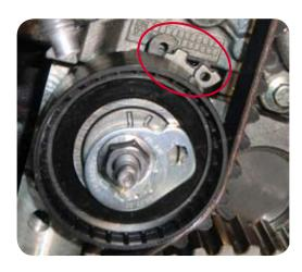
**6.** Fit the timing belt, ensuring that the marks on the belt align with the marks on the sprockets, then remove the locking pin from the tensioner. Rotate the tensioner anti-clockwise until pointer is at the position shown and **torque to 24 Nm**.
