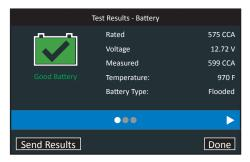
Test Results - Battery Test
