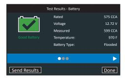
Test Results - Battery Test
