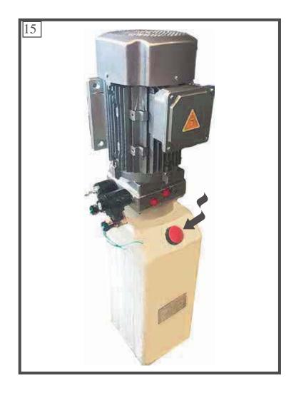
tank, completely disassemble the tank and empty out the remaining oil into the drain pan.
