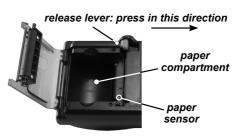
Place a new roll of paper in the compartment, and pull the paper forward so that it extends past the serrated edge of the paper slot.
