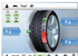
Concealed attachment of adhesive weights behind spokes
