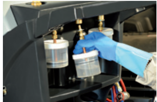
Hermetically closed oil and UV-dye bottles ensure moisture free and clean storage
