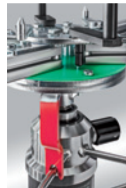
Safety latch (red) with rotary valve (black)
