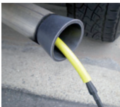
Leakfinder® can detect also leaks in the exhaust pipe system
